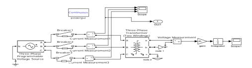
Fig8: Model with Sequential Switching Technique
