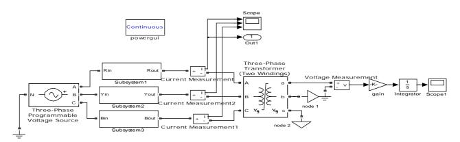
Fig 3: Model with Pre-insertion resistor method
