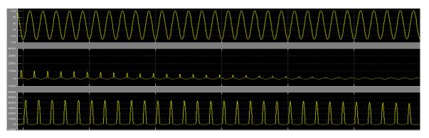
Fig 9: Current in phases R, Y and B of primary side with Sequential Switching method
