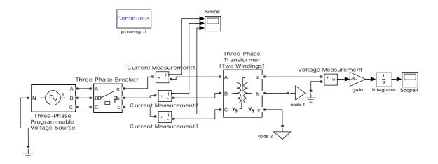
Fig. 1: Inrush Current Model without mitigation technique
